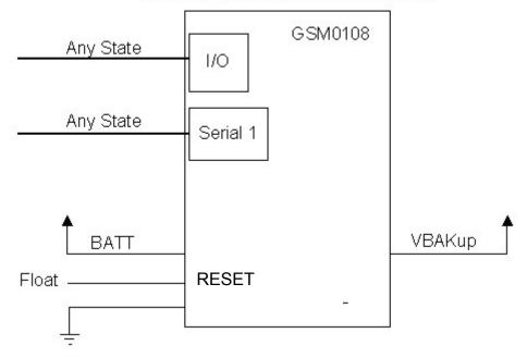
Figure 9 External Power Control Signal (no external processor)
